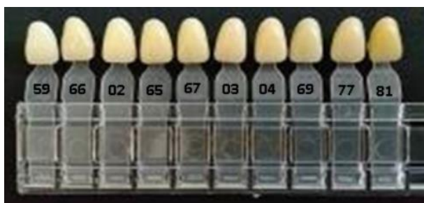
Figure 1: Visual measurement of stained acrylic teeth by using the Coral dental shade guide (from left to right: lighter to darker colours).
